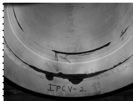
IPCV – Bush cracked
