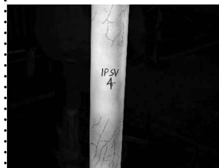
IPCV – Cracks on spindle
