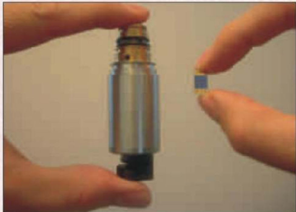
Fig 4 Standard Solenoid Valve and MEMS Micro valve
